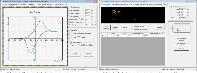
"4 Quadrant I-V" allows to plot Cyclic Voltammetry graphs.
