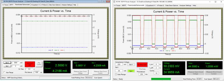
"Potentiostat/Galvanostat" tab allows user to use analyzer as Potentiostat or Galvanostat mode with given set voltage or set current value. Plotting V, I, and power also possible in this function. Programmable fix voltage or fix current On/Off timing function can use for electro deposition or lighting external laser diode with given on/off times and number of cycles.
