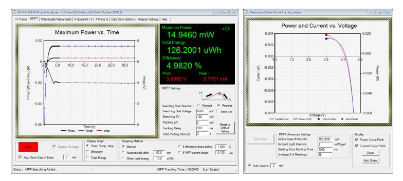
"MPP tracking" function shows the power, current, voltage and efficiency curves from the starting point of the MPP tracking so that user can see how it reach to maximum power point from different starting points and directions. It is continuously plot the conversion efficiency vs. tme curve.
