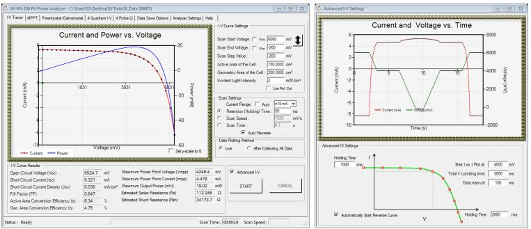
"Advanced IV Setup" allows user to change various settings such as "start" point holding time, "end" point holding time, current vs. time plot for each data point, and /or at given fixed voltage in the middle of I-V curve tracing.
